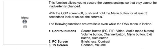
With the OSD screen off, push and hold the Menu button for five or more seconds to unlock the OSD settings.
